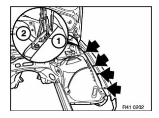
Unfasten upper retaining screws on side panel.
