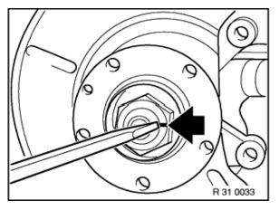
Peen down retainer on collar nut.
