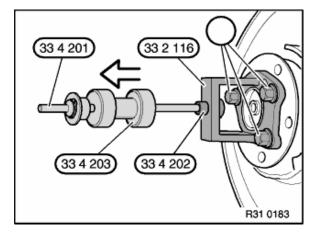
Pull off bearing unit with special tool 33 2 116 / 33 4 201 /202 / 203 and wheel studs (1).
