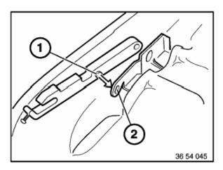
Setting lever with retaining screw:
