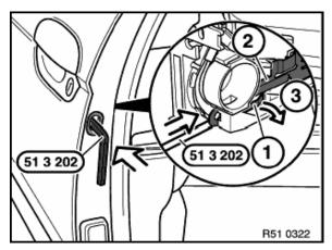
Insert special tool 51 3 202 and lever retaining tab (1) on locking plate (2) over the retaining lug (3).
