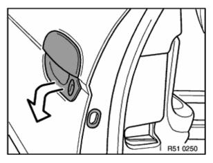
Insert special tool 51 3 201 in sliding bore on locking plate (2) and press locking plate forwards with raised retaining tab (1).
