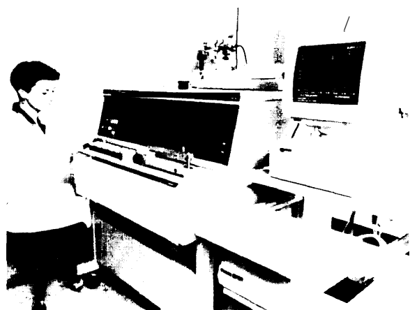
Costs of onsite inspection are one issue in assessing the net value of verification regimes for nonproliferation agreements. Pictured here is an x-ray fluorescence spectrometer used to analyze samples from nuclear inspections in Iraq.
