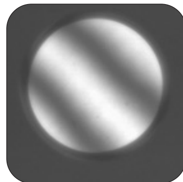
Bright and dark fringes of an interferogram.
