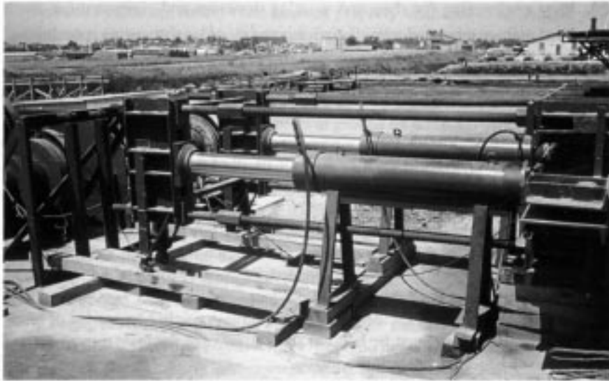
Long-stroke hydraulic jacks for stressing tendons.
